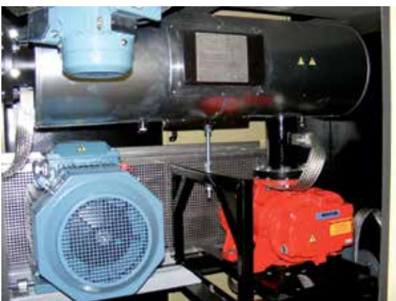
Package in version ATEX with acoustic enclosure
