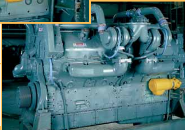
An ST650BP03R31 starter is shown mounted on a Detroit Diesel 12V-149R.
